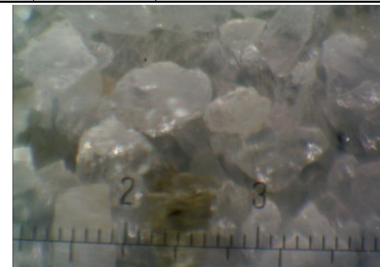
Photomicrograph of Lab ID 16110081-1 Arkansas White Bunker Sand.
